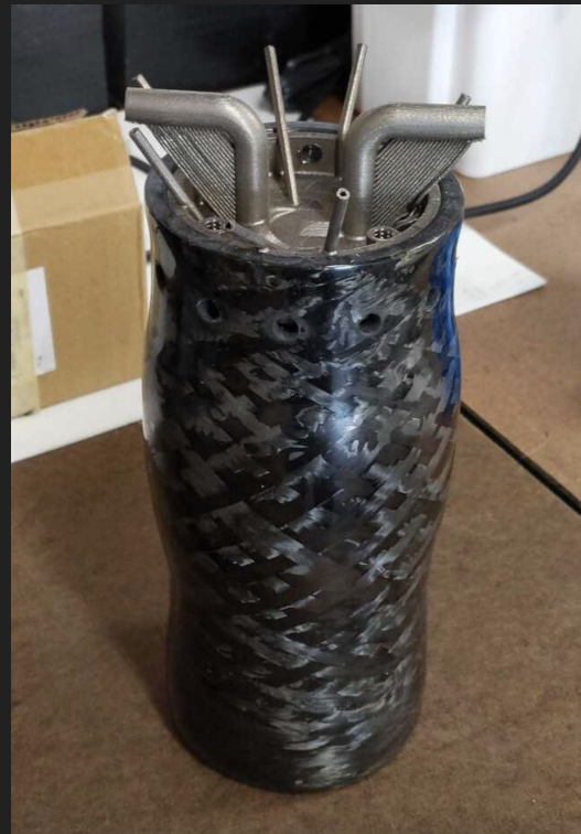
Above: Custom wound carbon fiber combustion chamber and 3D printed Inconel injector assembly.
